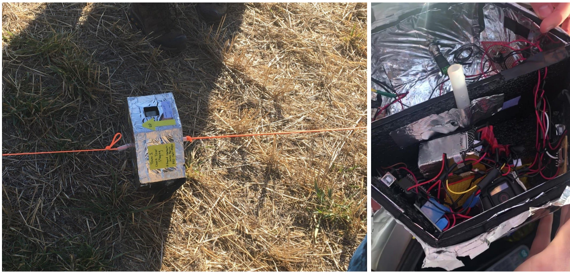
Figure 8.3.2 Exterior and interior of BalloonSat after recovery
